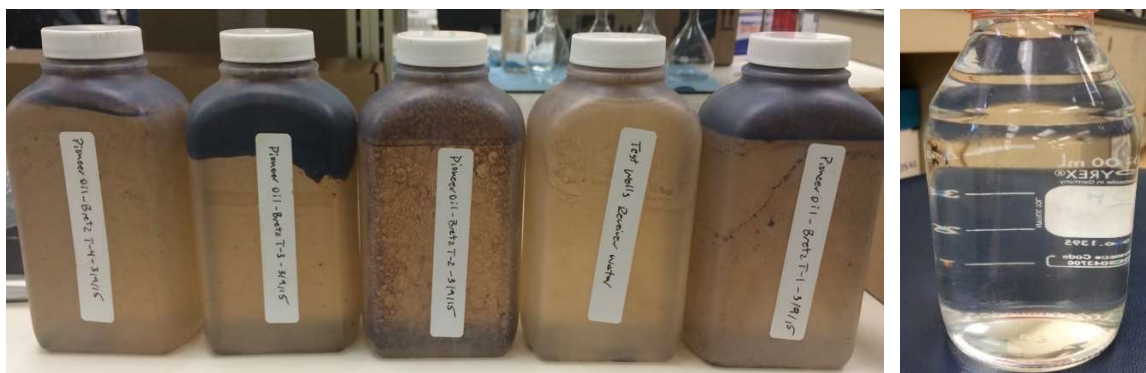
(a) Reservoir water samples capped with crude oil
