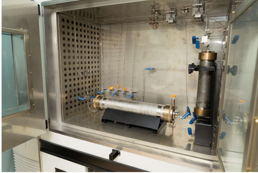
Figure 3.2 Core flood setup in Purdue's EOR lab
